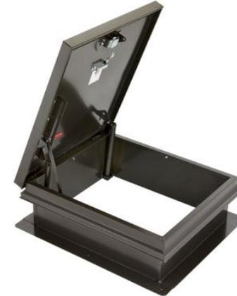
The Model RHA Series roof hatches provide for normal ladder, step ladder and stair access to roof from interior of the building. Manufactured from aluminum with weather resistant gasketing, these units feature long life, low maintenance and ease of operation. J.L. offers fully welded, mitered corners and box type door design. Units install easily over roof opening and are secured from base flange to roof deck.
