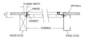
Model NGS met the performance criteria as per CSA A440-00 (windows) for an Air Infiltration of A-3 for both 75 Pa and 300 Pa, for Air Exinfiltration the sample met an A-3 rating at 75 Pa and A-2 rating at 300 Pa. In Water Tightness by Static Pressure the door sample met a B-1 rating, subject to using an optional watertight mechanism, phone for details
