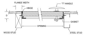
Model NWR met the performance criteria as per CSA A440-00 (windows) for an Air Tightness rating of A-3 at infiltration pressures of 75 Pa and 300 Pa and at exfiltration pressures of 75 Pa and 300 Pa. In Water Tightness by Static Pressure the door sample met a B-4 rating, subject to using an optional watertight mechanism, phone for details. Testing performed by Intertek (Warnock Hersey).
