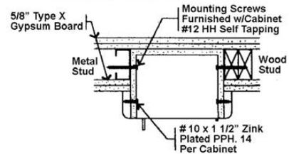
**WARNOCK HERSEY LISTED** UL Classified 5/8" Type X gypsum board inserted in the cavity between the two layers. Warnock Hersey has approved the Safeguard Cabinets to be mounted in any face of fire rated steel or wood stud for up to 2 hour rated walls without affecting its fire rating. The above meets the requirement test ASTM-E119-98 with test report WHI-495-1534. MOUNTING INSTRUCTIONS are supplied with each safeguard cabinet.
