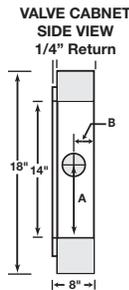
**SAFEGUARD Sonoma Series VC-SN Valve Cabinet Knockout Drilling:** No knockouts are provided with Sonoma Safeguard Valve Cabinets. Find the exact location of the pipe(s) which enter the cabinet and mark the cabinet tub appropriately. Both outside and inside tubs and insulation material must be completely open to receive pipe(s).
