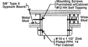
UL Classified 5/8" Type X gypsum board inserted in the cavity between the two layers. Warnock Hersey has approved the Safeguard Cabinets to be mounted in any face of fire rated steel or wood stud for up to 2 hour rated walls without affecting its fire rating. The above meets the requirement test ASTM-E119-98 with test report WHI-495-1534. MOUNTING INSTRUCTIONS are supplied with each Safeguard cabinet.
