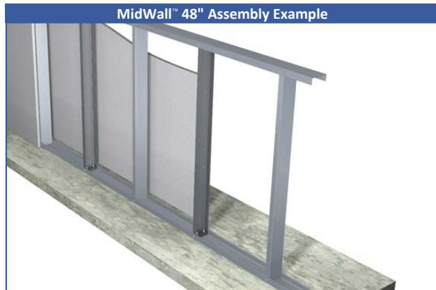
MidWall 48" is used in interior half walls equal to or more than 48" in height. Use one MidWall 48" as a substitute for a stud at the specified spacing, or attach to a 54mil stud with #12 screws through all pre-drilled guide holes. Maximum spacing between MidWall connectors is 36" o.c.
