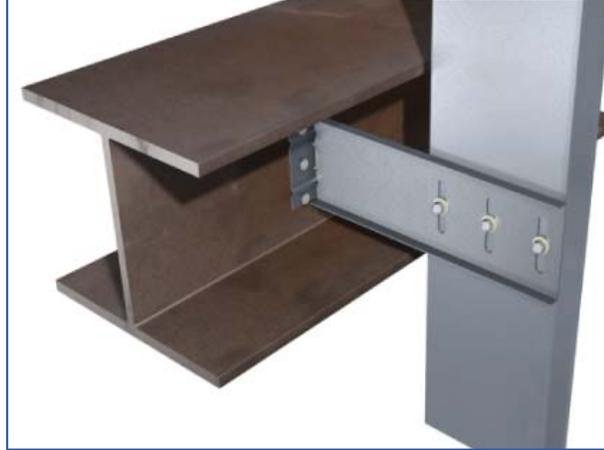
Standard offset of stud from the heel of the clip should not exceed 1.0". Step Bushings and Screws may be installed in the middle and outer slots of SLB600 or 800 to accommodate greater building tolerances. Note that this may affect the F1 and F2 allowable load capacity and may require a row of bridging at a maximum distance of 12" of the connection to resist stud torsional effects. Call TSN Tech Support for test data and recommendations.
