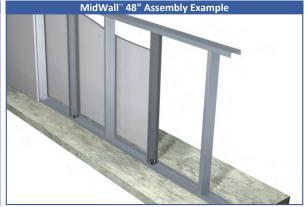
MidWall 24" is generally used in interior half walls of less than 48" MidWall 48" is used in interior half walls equal to or more than MidWall connectors is 36" o.c.
