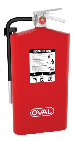
**Application:** Multi-purpose 10 lb. dry chemical fire extinguisher for wall and cabinet mounting. For use on Class A, B and C fires. Not recommended for use on sensitive electronic equipment.
